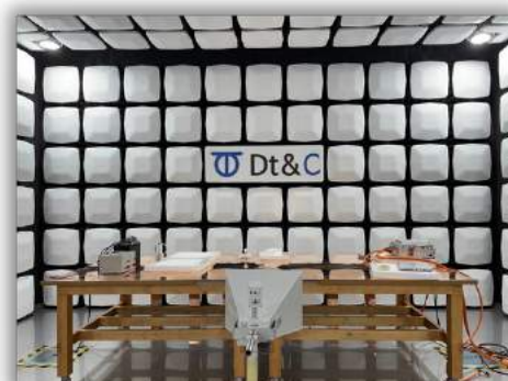
Absorber lined Shielded Enclosure (EMI/EMS Chamber: 1 system)
